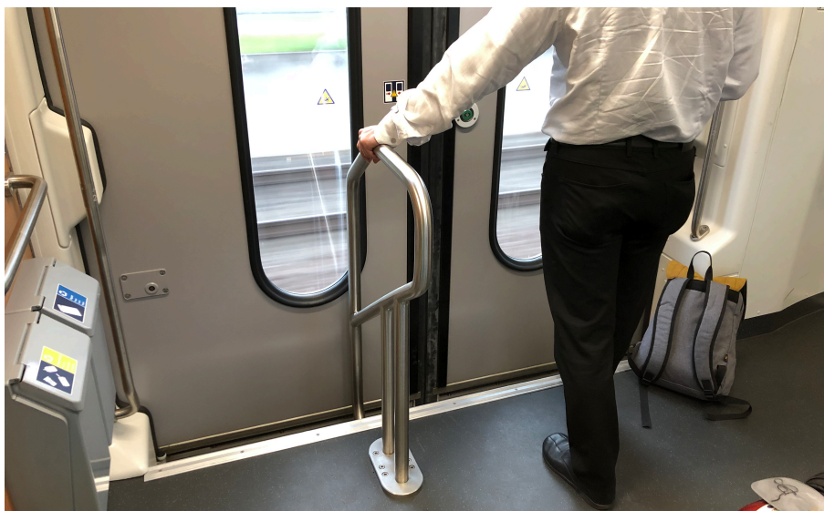
Fig 11 – A handrail not aligned to the center of the train door
