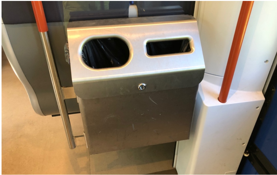
Fig 10 – Trash cans in the train using different geometric shapes for trash sorting
