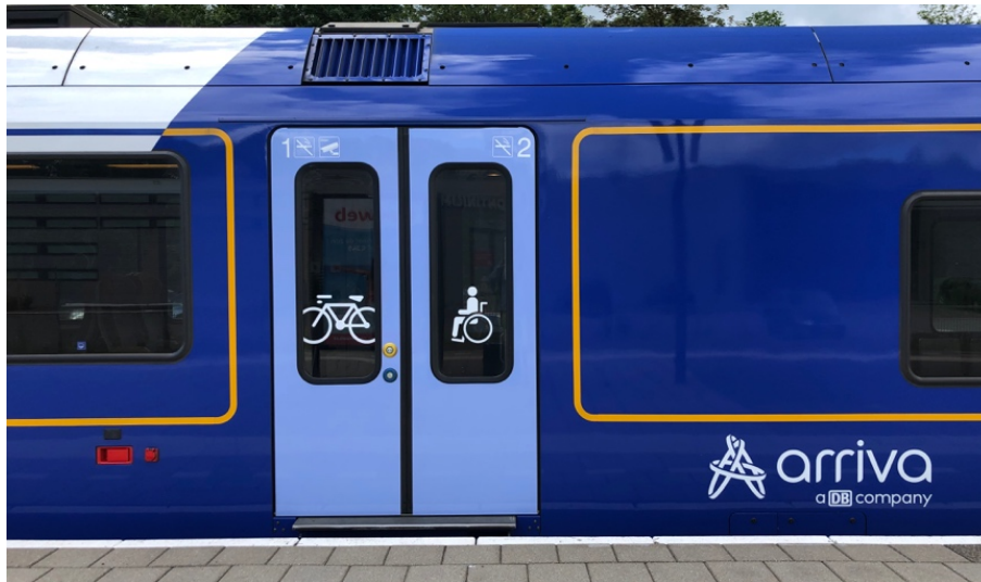
Fig 12 – An exterior sign clearly indicating that the carriage is designed for passengers with bikes or limited physical mobility
