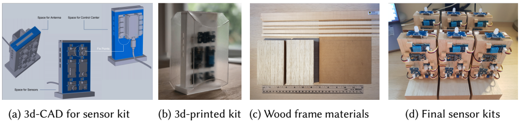
Fig. 2. The overall production process of our smart home sensor kits
