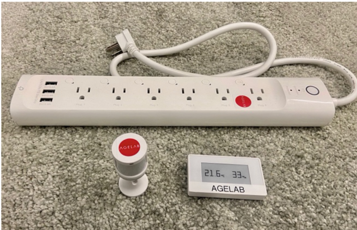
Fig. 9. Selected hardware for version 2 of the kit. Wifi-enabled power strip (top), Zigbee-enabled motion sensor (bottom left), and Zigbee-enabled air quality monitor (bottom right).
