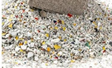
Yi Design turns ceramic waste into waterpermeable bricks
